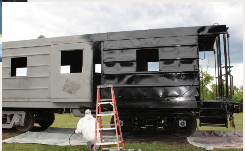
Doug Peterson begins to apply the epoxy primer to the caboose as a protective coating
