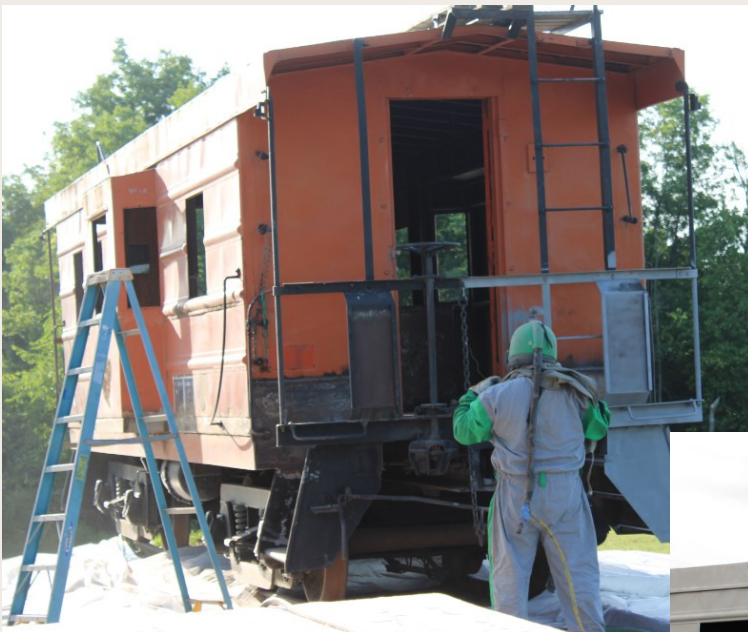
Doug Peterson begins to apply the epoxy primer to the caboose as a protective coating
